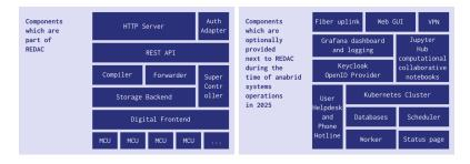
Fig. 13.1: Overview about the REDAC-internal services vs. the services operated by anabrid. Click to enlarge.
